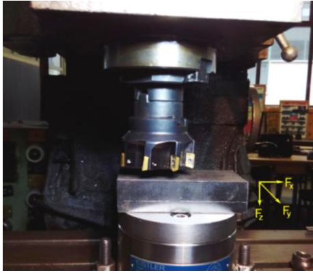
Fig. 2 – Cutting force measurement system.
